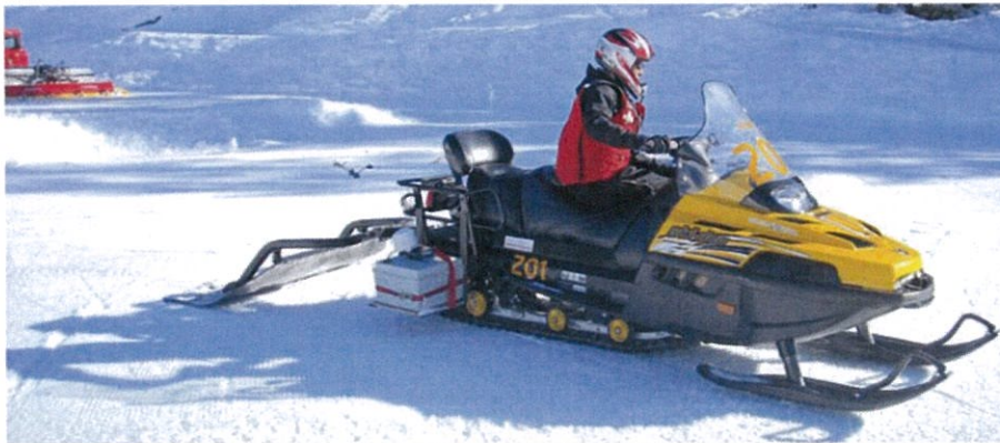
Temperature mapping methods used to collect snow surface temperature data along the 2010 Olympic cross-country ski racing courses. A snowmobile was used to carry the instrumentation along the 10km racing tracks.
