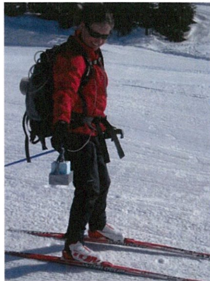
The author generating a temperature map along the 2.4km representative course using the instrumentation. The equipment was inside a backpack and the infrared sensor held out to the side
